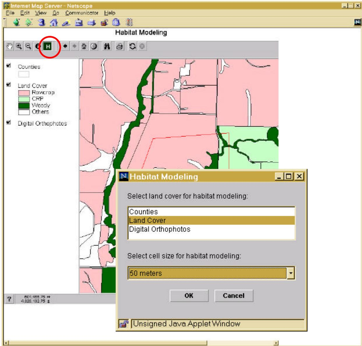
Figure 3. Use habitat model tool to define a study area and select land cover data layer and grid cell size
